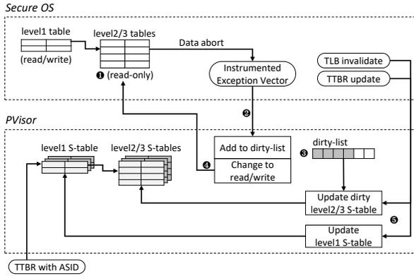
Fig. 8: The page table virtualization of PrOS based on the shadow paging.
