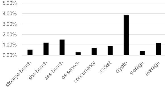
Fig. 10: Performance Overhead of `xtest`. The suffix "bench" means that the associated test group performs a stress test.
