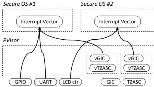
Fig. 9: Assignment and emulation for device virtualization.
