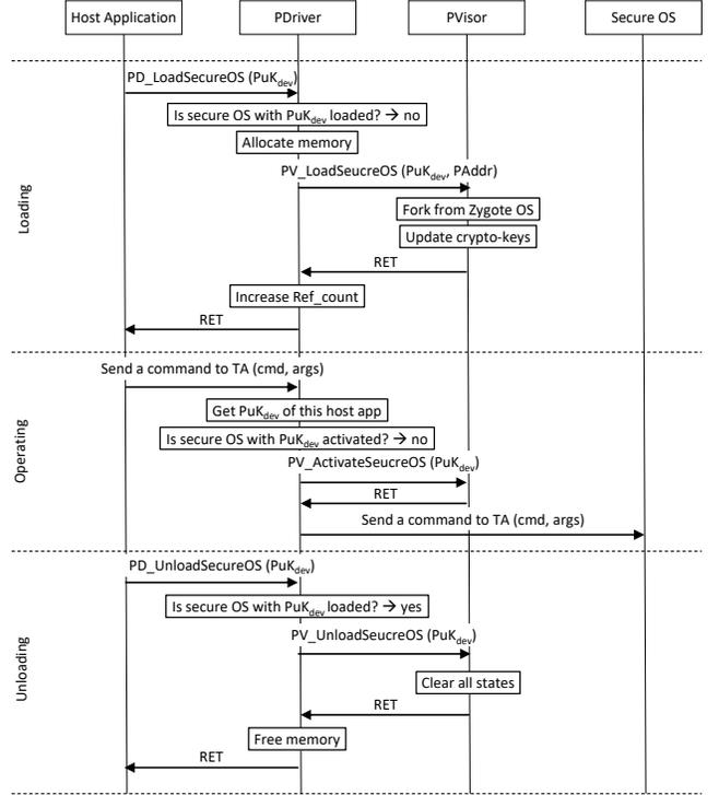
Fig. 6: The workflow of host application with PrOS.
