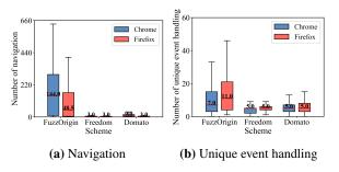
**Figure 6:** The number of navigation completion and unique event handling for a single fuzzing iteration by each scheme. In both cases, FUZZORIGIN achieved the highest number.
