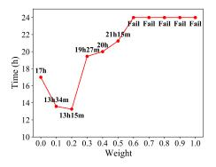
**Figure 8:** An elapsed time in average to detect seven previously known CVEs while varying WEIGHTED\_RAND. When WEIGHTED\_RAND is higher than 0.6, no CVEs were found within 24 hours of running.
